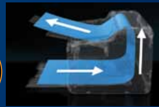
A short paper path enables smooth printing and prevents paper from getting stuck.
